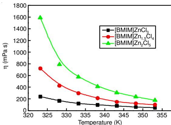
Fig. 4. Viscosity of ionic liquids at temperature from 323.15-353.15 K
