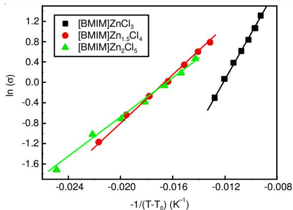
Fig. 3. Relationship between conductivity and temperature based on VFT equation
