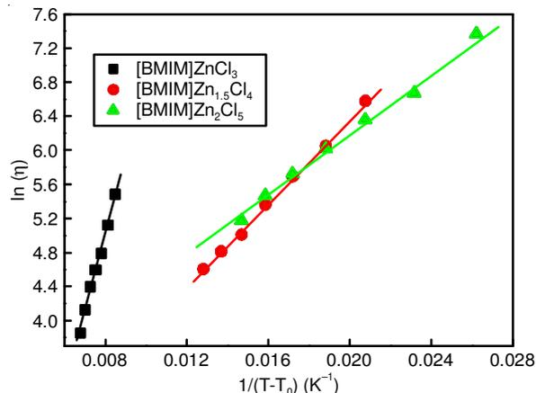
Fig. 6. Relationship between viscosity and temperature based on VFT equation
