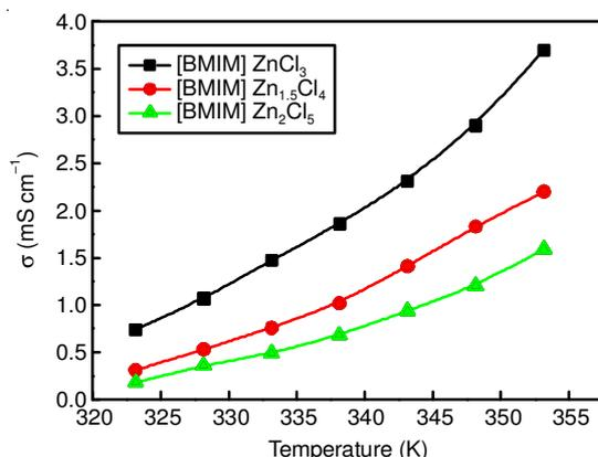
Fig. 1. Conductivity of ionic liquids at temperature from 323.15-353.15 K
