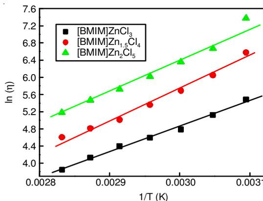
Fig. 5. Relationship between viscosity and temperature based on Arrhenius equation
