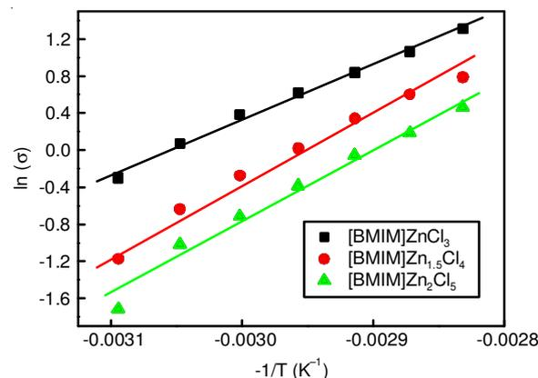
Fig. 2. Relationship between conductivity and temperature based on Arrhenius equation
