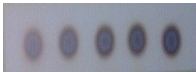
Fig. 4. Hydrogen per oxide determination by Iodide
