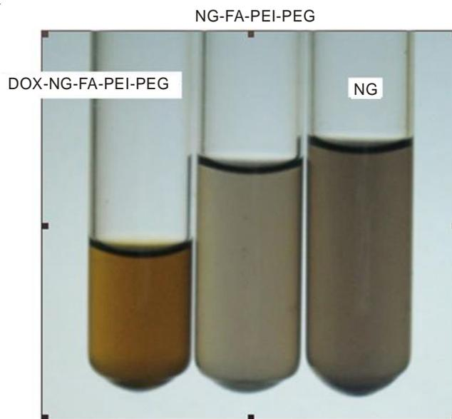
Fig. 2. Aqueous solution of nano graphene, NG-FA-PEI-PEG and DOX-NG-FA-PEI-PEG
