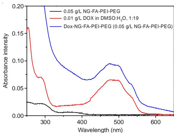
Fig. 9. UV-visible spectra of DOX, NG-FA-PEI-PEG and Dox-NG-FA-PEI-PEG
