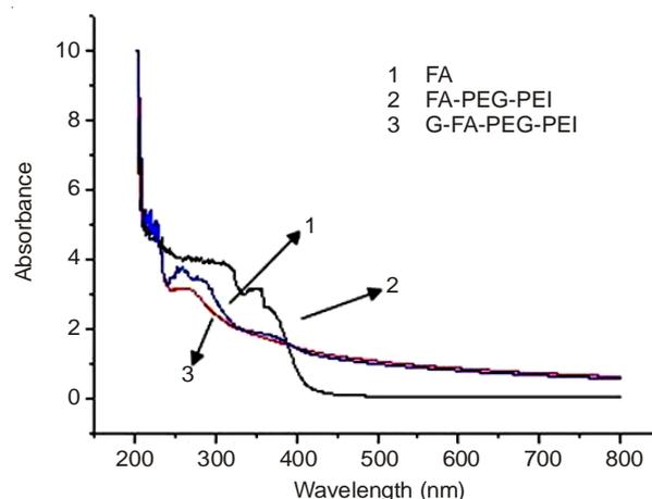
Fig. 8. UV-visible spectra of the folic acid, FA-PEG-PEI and G-FA-PEG-PEI in aqueous solution
