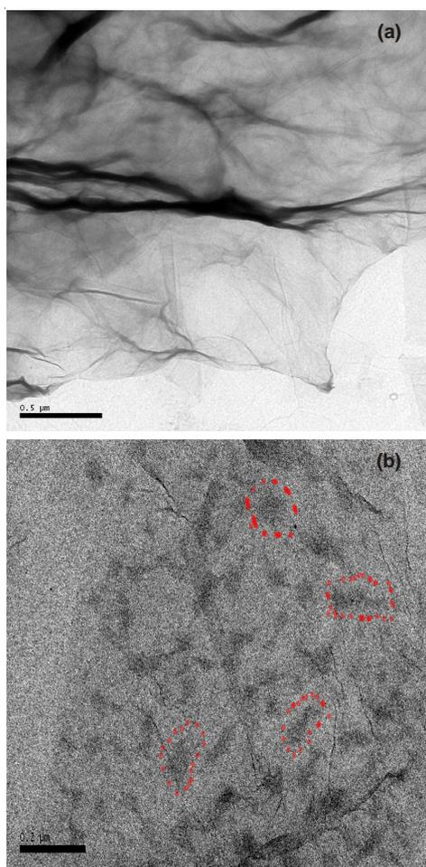
Fig. 6. TEM microscopy of big pieces reduced graphene oxide (a); the small pieces reduced graphene oxide which were obtained by sonication (b)
