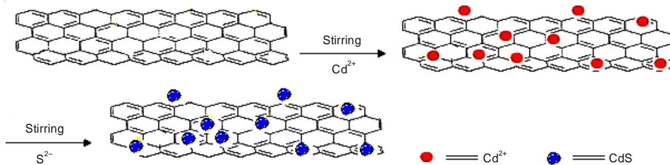
Fig. 3. Schematic illustration of CdS-NG-FA-PEI-PEG preparation (Here, FA-PEI-PEG no displayed)
