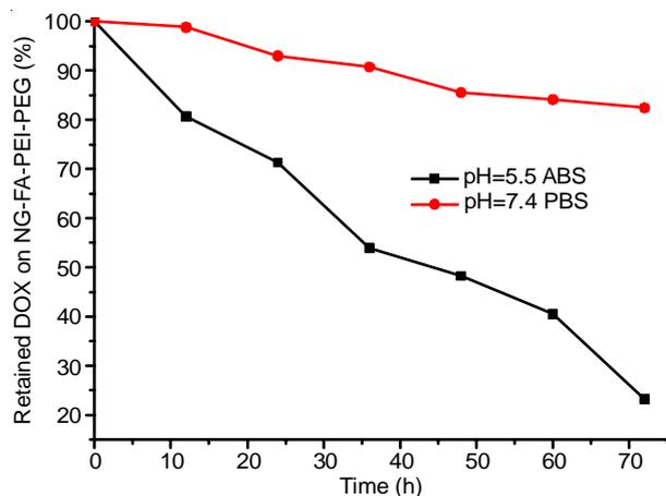
Fig. 10. Correlation plot of retained doxorubicin on reduced graphene oxide sheets with time increasing in different pH solution
