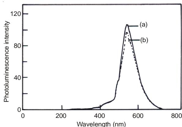
Fig. 1. Photoluminescence emission spectrum of phenothiazinophane **5** in  $CHCl_3$  ( $1 \times 10^{-5}$  M) (a)  $CHCl_3$  medium. (b)  $CHCl_3$  and TFA (pH = 5)
