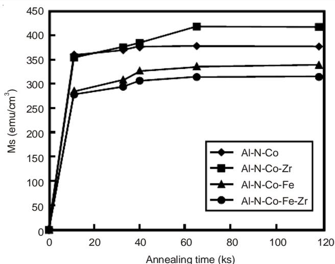
Fig. 3. Variations of saturation magnetization as a function of annealing time for Al-N-Co-(Zr/Fe/Zr-Fe) films annealed at 773 K for 118.8 ks
