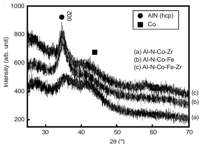
Fig. 1. Typical XRD profiles of as-deposited Al-N-Co-(Zr/Fe/Zr-Fe) films
