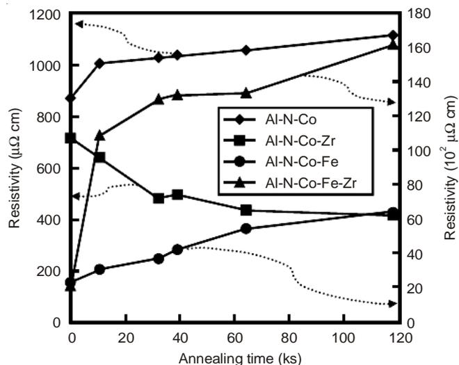
Fig. 4. Variations of resistivity as a function of annealing time for Al-N-Co-(Zr/Fe/Zr-Fe) films annealed at 773 K for 118.8 ks
