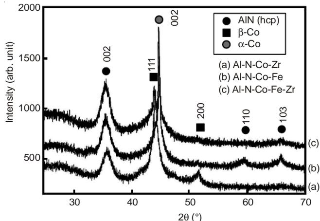
Fig. 2. Typical XRD profiles of Al-N-Co-(Zr/Fe/Zr-Fe) films annealed at 773 K for 118.8 ks
