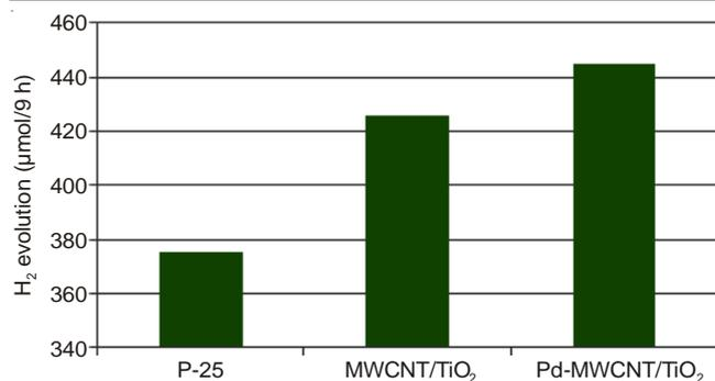
Fig.3. Photocatalytic H<sub>2</sub> evolution of as-prepared samples and P-25 using Na<sub>2</sub>S/Na<sub>2</sub>SO<sub>3</sub> as sacrificial reagent
