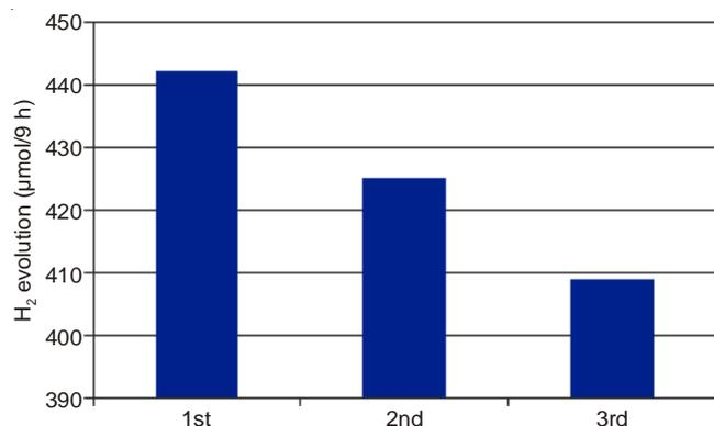
Fig. 5. Cyclic test of Pd-MWCNT/TiO<sub>2</sub> nanocomposite using Na<sub>2</sub>S/Na<sub>2</sub>SO<sub>3</sub> as sacrificial reagent under UV light irradiation
