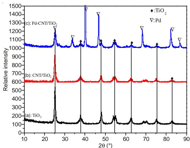
Fig. 1. XRD patterns of pure anatase TiO<sub>2</sub> (a), MWCNT/TiO<sub>2</sub> (b) and Pd-MWCNT/TiO<sub>2</sub> (c).
