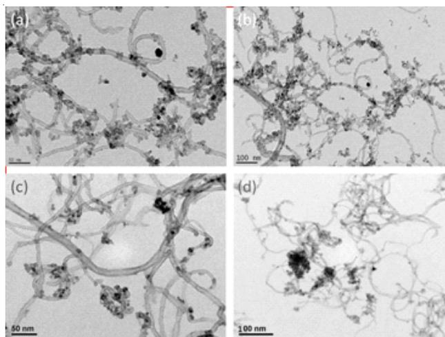
Fig. 2. TEM images of composite photocatalysts: (a)&(b) MWCNT/TiO<sub>2</sub>, (c)&(d) Pd-MWCNT/TiO<sub>2</sub>
