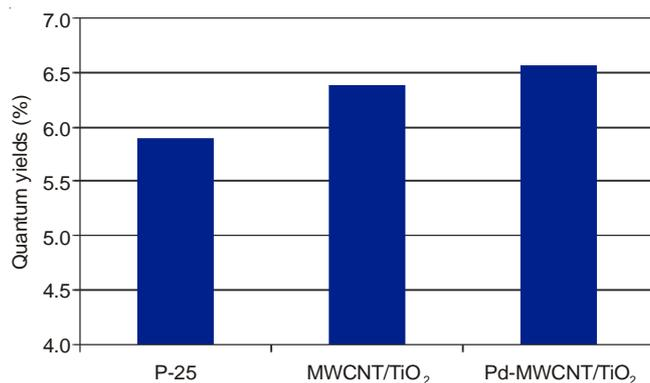
Fig. 4. Quantum yields for hydrogen evolution by as-prepared samples and P-25 with Na<sub>2</sub>S/Na<sub>2</sub>SO<sub>3</sub> aqueous solution
