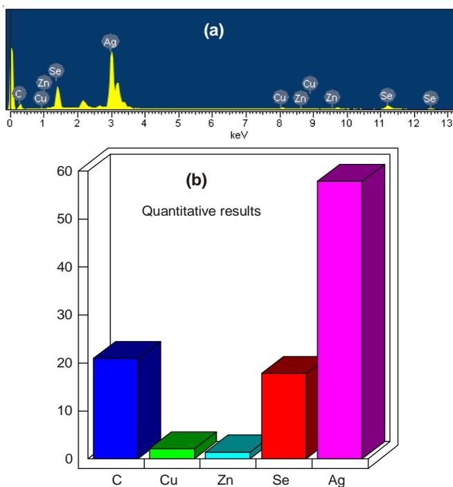
Fig. 3. EDX microanalysis (a) and element weight % (b) of  $\text{Ag}_2\text{Se}$ -graphene composite
