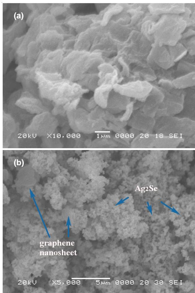
Fig. 2. SEM images of as-prepared composites: (a) GO, (b) Ag<sub>2</sub>Se-graphene composite
