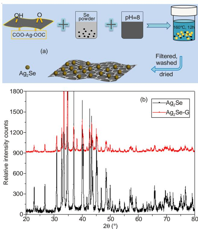
Fig. 1. (a) Schematic illustration of deposition of Ag<sub>2</sub>Se on the graphene, (b) XRD pattern of Ag<sub>2</sub>Se and Ag<sub>2</sub>Se-graphene composite
