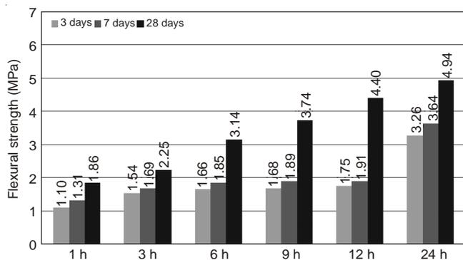
Fig. 8. Flexural strength based on variation of water curing time at 80 °C
