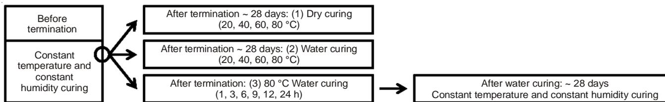
Fig. 1. Curing method
