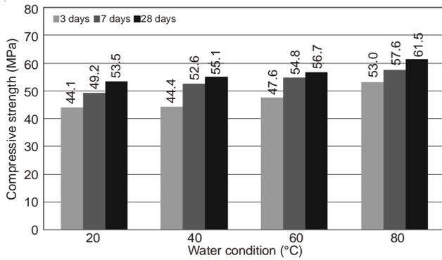
Fig. 5. Compressive strength by water curing temperature
