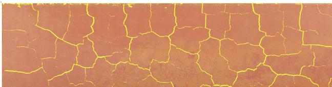
Fig. 6. Crack in matrix during the dry curing at 80 °C
