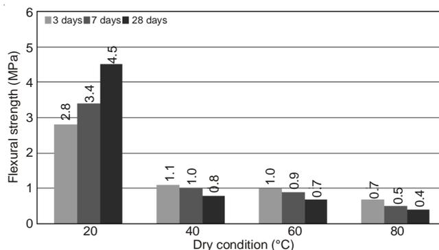
Fig. 3. Flexural strength by dry curing temperature
