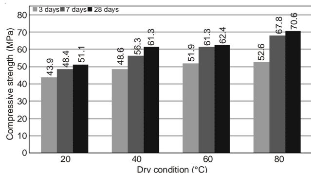
Fig. 2. Compressive strength by dry curing temperature
