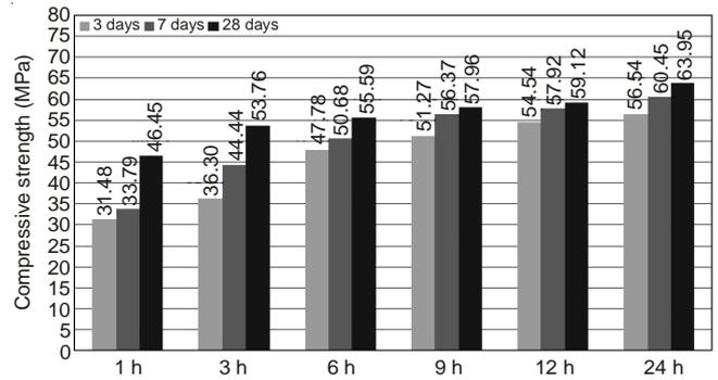
Fig. 9. Compressive strength based on variation of water curing time at 80 °C
