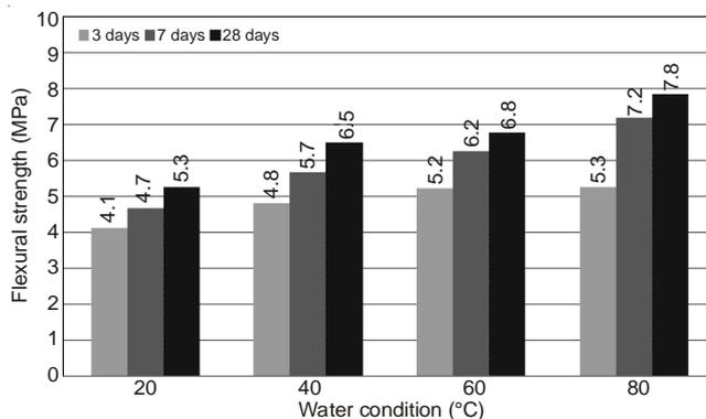
Fig. 4. Flexural strength by water curing temperature
