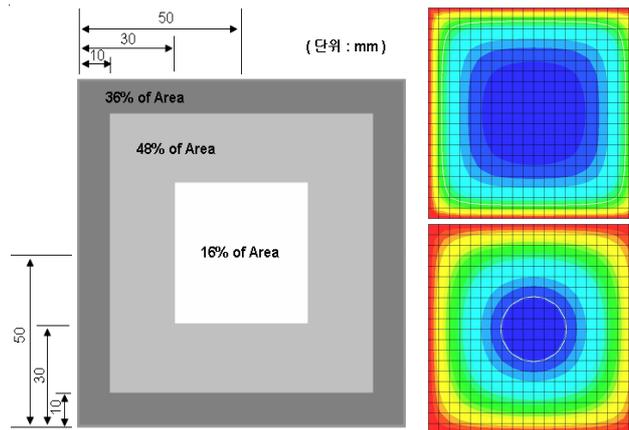
Fig. 2. Calculation of temperature distribution
