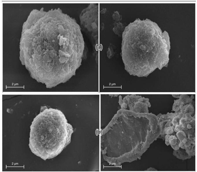
Fig. 6. FE-SEM photographs of (a) MC-GO (b) MC-GO-Ser
