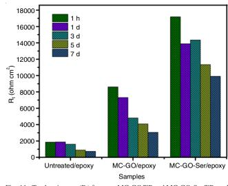
Fig. 11. Total resistance (Rt) for neat, MC-GO/EP and MC-GO-Ser/EP steel samples
