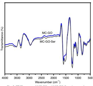
Fig. 5. FT-IR spectra of MC-GO and MC-GO-Ser microcapsules
