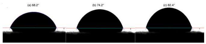
Fig. 13. Contact angle values of (a) neat EP, (b) MC-GO/EP and (c) MC-GO-Ser/EP coatings
