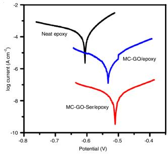
Fig. 8. Polarization curves of epoxy coated samples after 7 d exposure in corrosion solution
