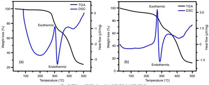
Fig. 7. TGA and DSC plots of (a) MC-GO (b) MC-GO-Ser
