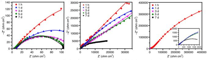
Fig. 10. Nyquist plots of neat EP, MC-GO/EP and MC-GO-Ser/EP coated samples
