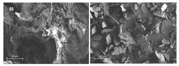
Fig. 3. FE-SEM images of (a) GO and (b) GO-Ser
