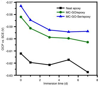
Fig. 9. OCP curves of neat EP, GO/EP and GO-Ser/EP coatings after 7 d
