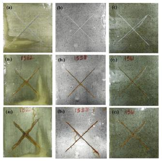
Fig. 12. Salt spray test results of (a) neat EP (b) MC-GO/EP (c) MC-GO-Ser/EP after 7 d and 14 d
