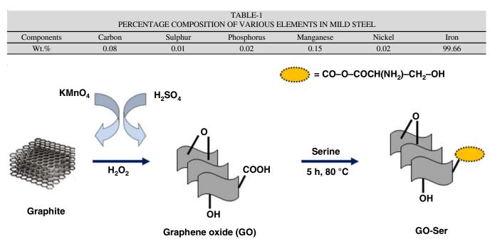
Fig. 1. Schematic diagram describing the preparation of GO-Ser
