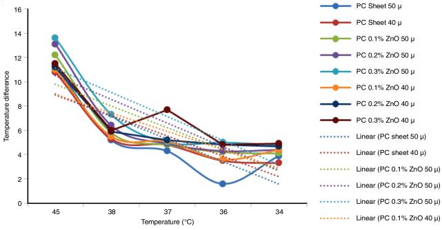
Fig. 4. Effect of temperatures on 50 & 40 µ thickness of polycarbonate (PC) coated ZnO sheets
