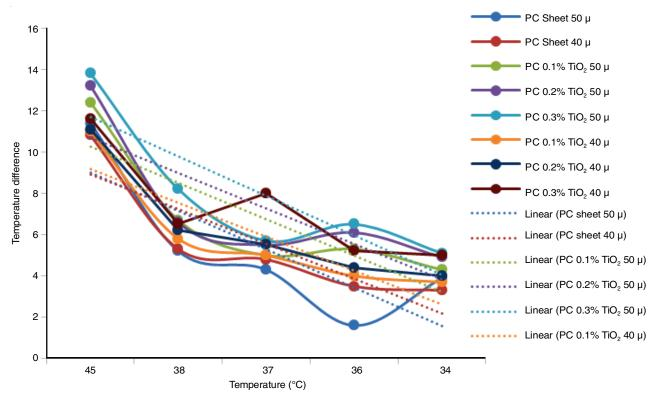
Fig. 5. Effect of temperatures on 50 and 40 µ thickness of polycarbonate (PC) coated TiO<sub>2</sub> sheets
