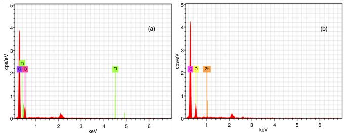
Fig. 3. EDS spectrum of polycarbonate (PC) coated 0.3% TiO<sub>2</sub> (a) and polycarbonate (PC) coated 0.3% ZnO (b) nanosheets
