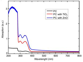
Fig. 2. UV-vis spectra of polycarbonate (PC) (a); PC coated 0.3% TiO<sub>2</sub> (b); and PC coated 0.3% ZnO (c) nanosheets
