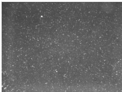
Fig. 1. (c) PLM of isotactic polypropylene with 0.2 wt. % nucleating agent DHDBS
