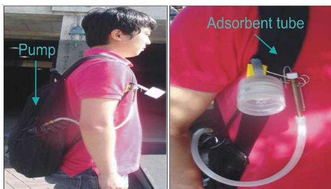
Fig. 2. View of the personal monitoring samplers
