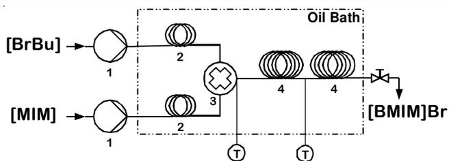
1. Syringe pump; 2. preheating coil; 3. micromixer; 4. delay pipe
