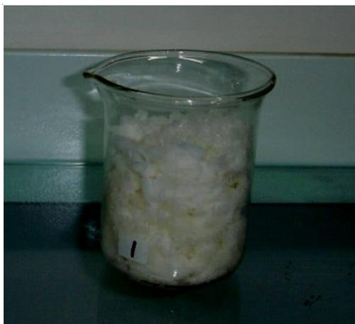
Fig. 7. Photo of obtained ionic liquid [BMIM]Br (synthesis condition: 1:1.05, 105 °C, and 3.2 min)
