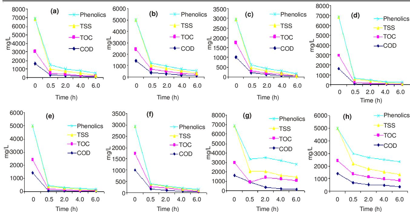
Fig 2. Time dependent effect of various advanced oxidation processes on phenolic, TSS, TOC, COD: (a), (b) and (c) Fenton treatment of Kalash Textile Mill (MTM), Kalash and Noor Fatima effluents, (d), (e) and (f) Photo fenton treatment of MTM, Kalash and Noor Fatima effluents, (g) and (h) Potassium permanganate treatment of MTM and Kalash effluent
