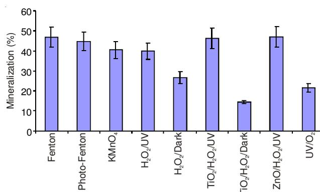
Fig. 1. Effect of various treatments on mineralization (%) of textile effluents (n = 3)
