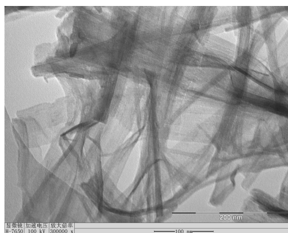
Fig. 2. (a) XRD pattern, (b) TEM image of the as prepared ultrathin BiOCl nanosheets
