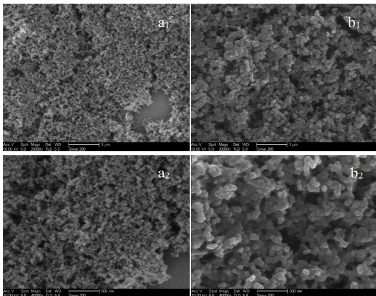
Fig. 3. SEM of original SiO<sub>2</sub> nanoparticles (a<sub>1</sub>, 20,000 times, a<sub>2</sub>, 40,000 times) and functionalized SiO<sub>2</sub> nanoparticles (b<sub>1</sub>, 20,000 times, b<sub>2</sub>, 40,000)
