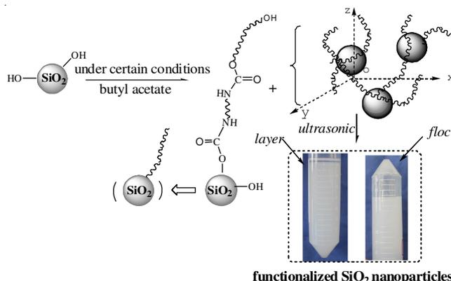
**Scheme-I:** Preparation route of functionalized SiO<sub>2</sub> nanoparticles
