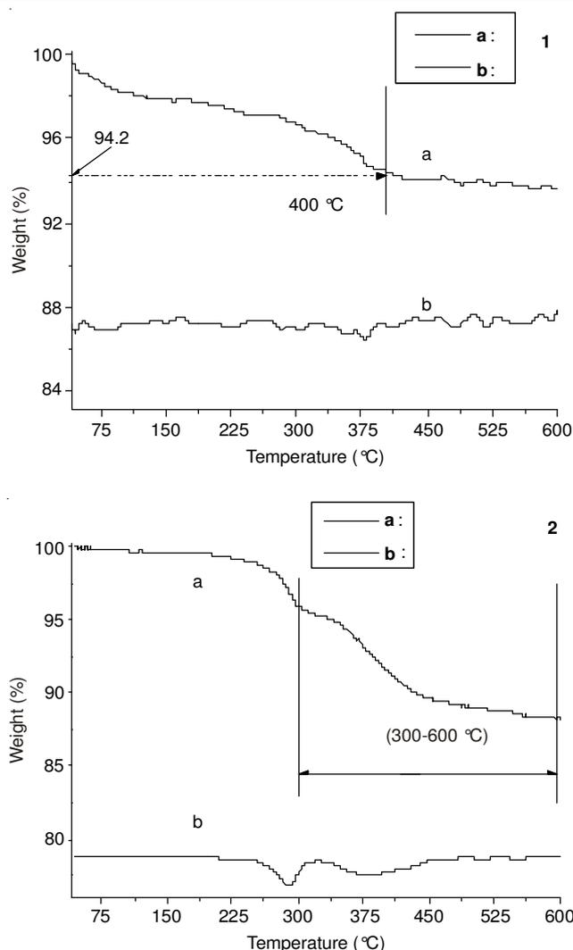
Fig. 2. (1) the original SiO<sub>2</sub> nanoparticles (a. TGA curves, b. DTG differential curve); (2) functionalized SiO<sub>2</sub> nanoparticles (a. TGA curves, b. DTG differential curves)
