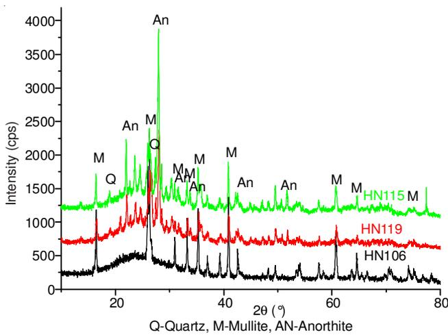
Fig. 3. XRD results of three Huainan coal ashes at 135 °C in reducing condition
