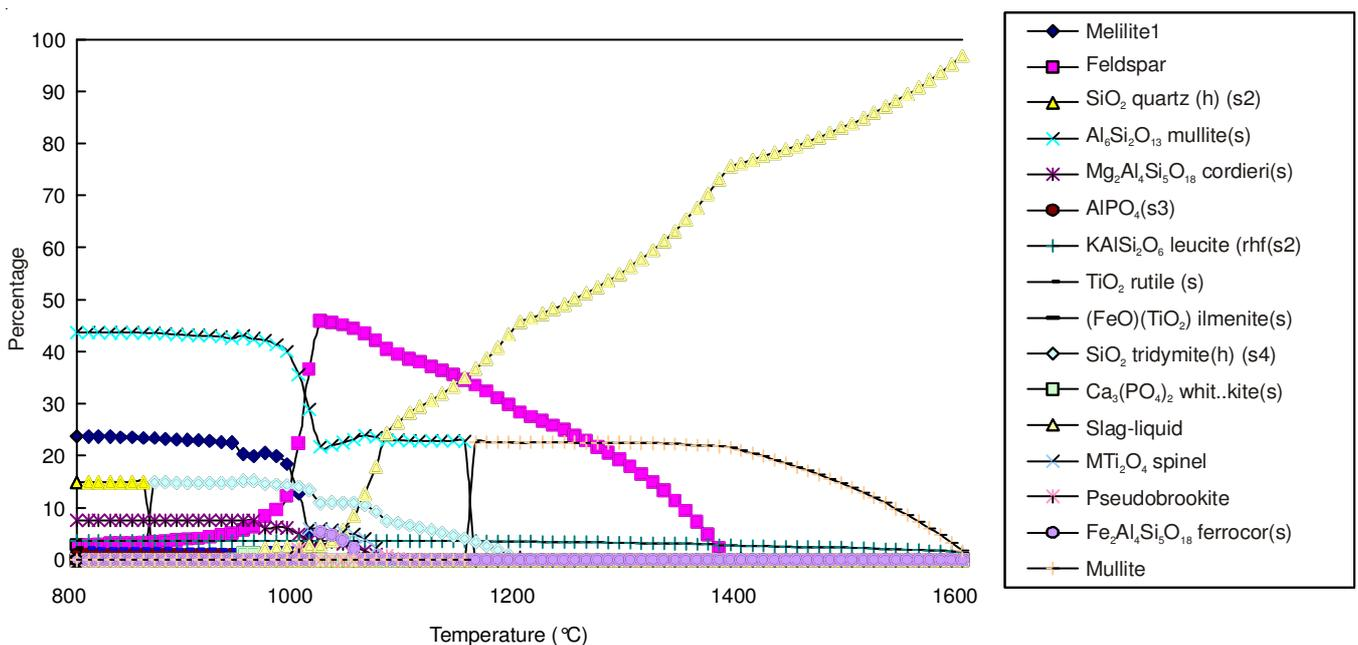
Fig. 5. Phase change of HN115 coal ash under reducing condition
