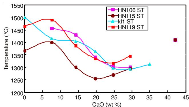
Fig. 7. Effect of CaO addition on the ash fusion temperature of Huainan coals
