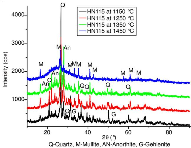
Fig. 2. XRD patterns of HN115 coal ash at different temperature under reducing atmosphere
