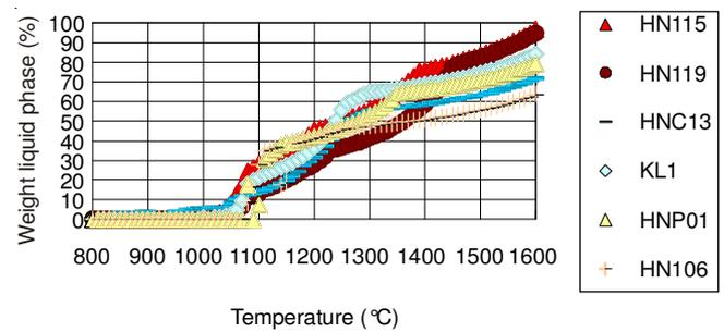
Fig. 4. Weight per cent of liquid phase for representative Huainan coal ash samples
