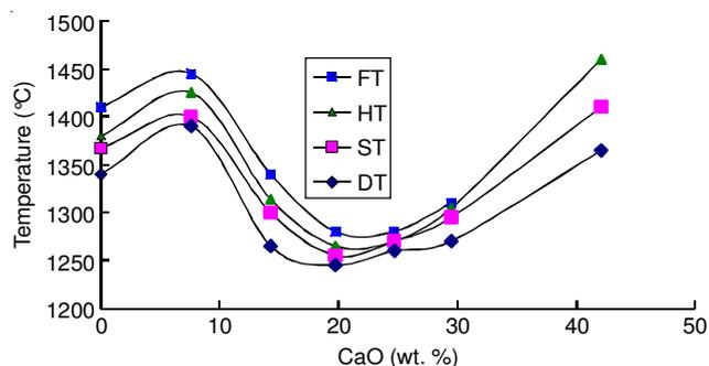
Fig. 6. Effect of CaO on the HN115 coal ash fusion temperature
