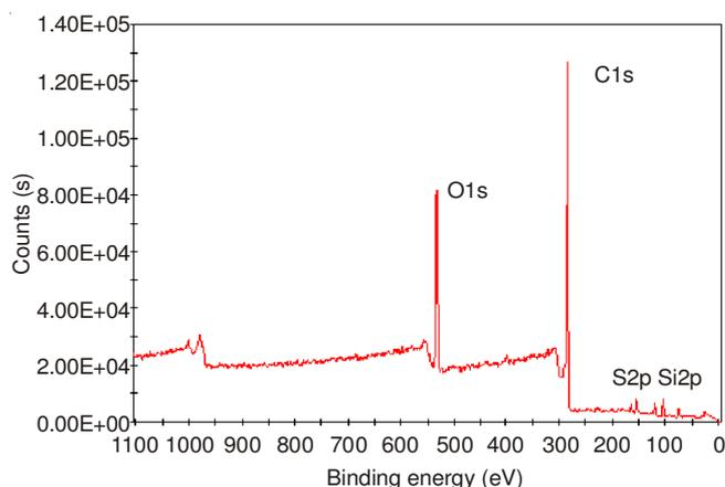
Fig. 1. XPS spectrum in the sample coal
