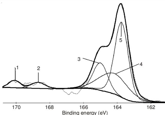
Fig. 4. XPS fitting spectrum of S2p
