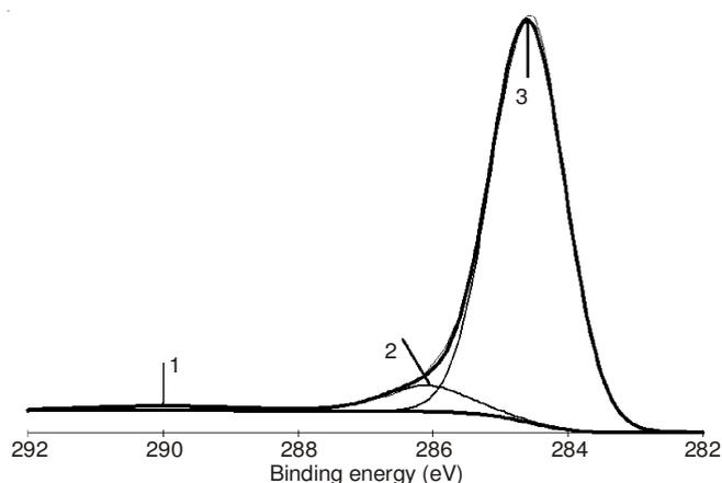
Fig. 2. XPS fitting spectrum of C1s
