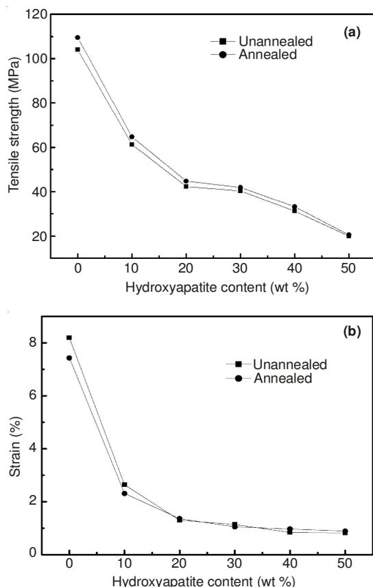
Fig. 2. Annealed and unannealed tensile strength (a) and strain (b) of nano-HA/PEEK FGM showing the effects of different levels of hydroxyapatite reinforcement at 10 HCDBAL
