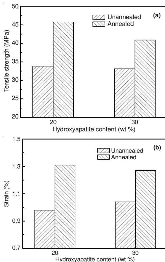
Fig. 3. Representative tensile strength-hydroxyapatite content(a) and strain-hydroxyapatite content (b) for tensile tests of annealed and unannealed PEEK FGM reinforced with 20 and 30 wt % hydroxyapatite nano-powder at 20 HCDBAL
