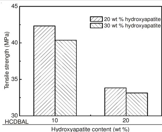
Fig. 4. Tensile strength of the unannealed PEEK functional gradient biocomposites reinforced with 20 and 30 wt. % hydroxyapatite nano-powder at 10 and 20 HCDBAL
