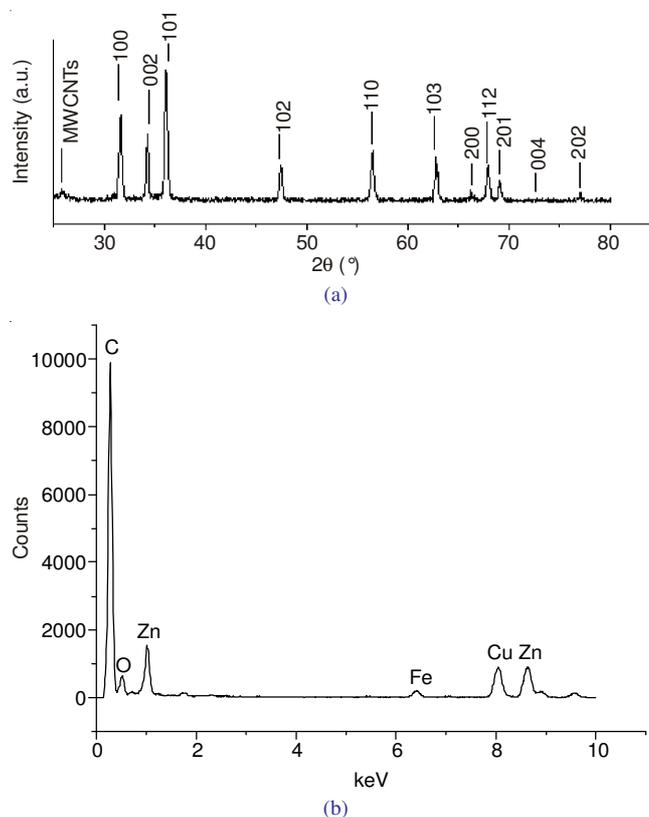
Fig. 1. XRD (a) and EDS (b) patterns of MWCNTs/Fe(III)/ZnO
