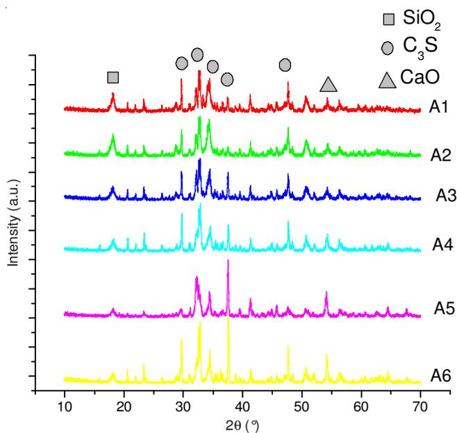
Fig. 2. XRD of  $C_3S$  samples with different content of both ZnO and CuO combined
