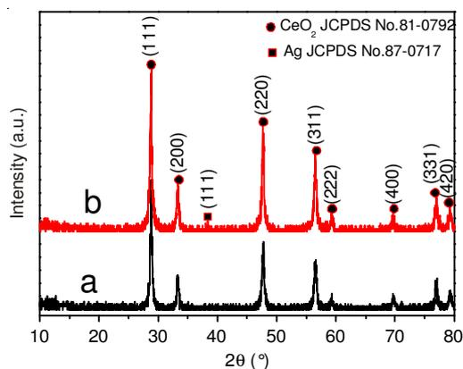
Fig. 1. XRD pattern of (a) mesoporous  $\text{CeO}_2$  and (b)  $\text{Ag}/\text{CeO}_2$  mesoporous composite
