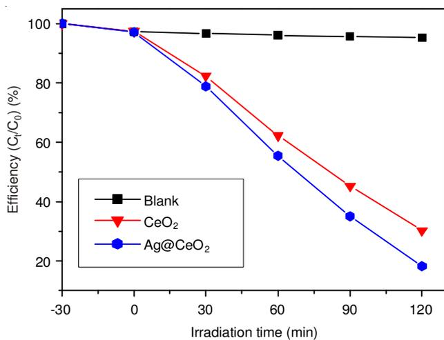
Fig. 4. Photodegradation efficiency of methylene blue under visible light irradiation over different conditions
