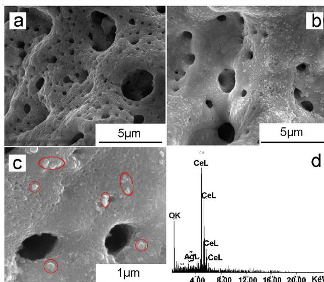
Fig. 2. (a) SEM images of mesoporous  $\text{CeO}_2$ , (b and c) SEM images with low and high magnification of  $\text{Ag}/\text{CeO}_2$  mesoporous composite, (d) EDX spectrum of  $\text{Ag}/\text{CeO}_2$  mesoporous composite
