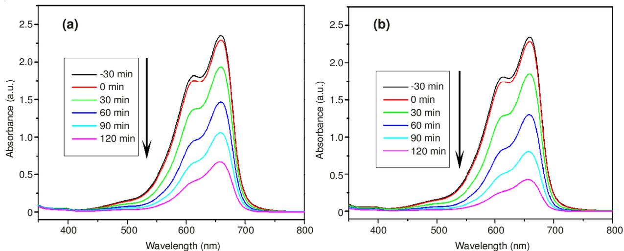
Fig. 3. Evolution of the absorption spectrum of methylene blue solution ( $5 \times 10^{-5}$  mol/L, 100mL) in the presence of (a) mesoporous CeO<sub>2</sub> and (b) Ag/CeO<sub>2</sub> mesoporous composite under visible light irradiation
