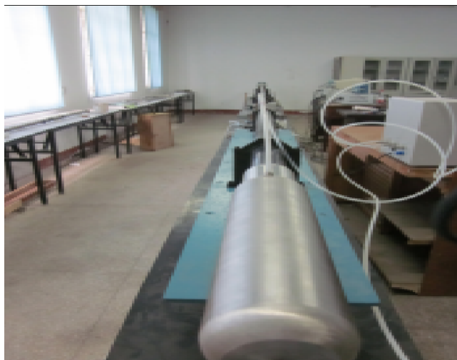
Fig. 2. Split Hopkinson pressure bar system
