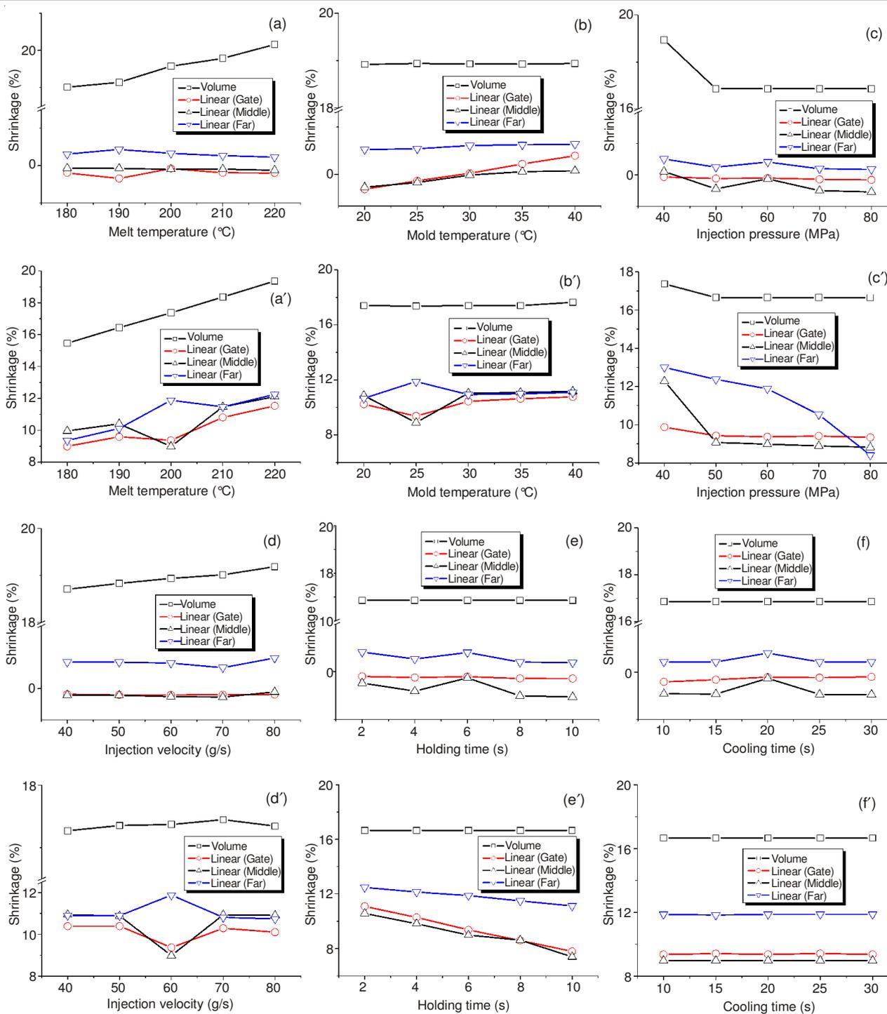
Fig. 1. Effect of operational variables on the shrinkage of PLA1. Thickness of cavity: (a-f) 1 mm, (a'-f') 4 mm
