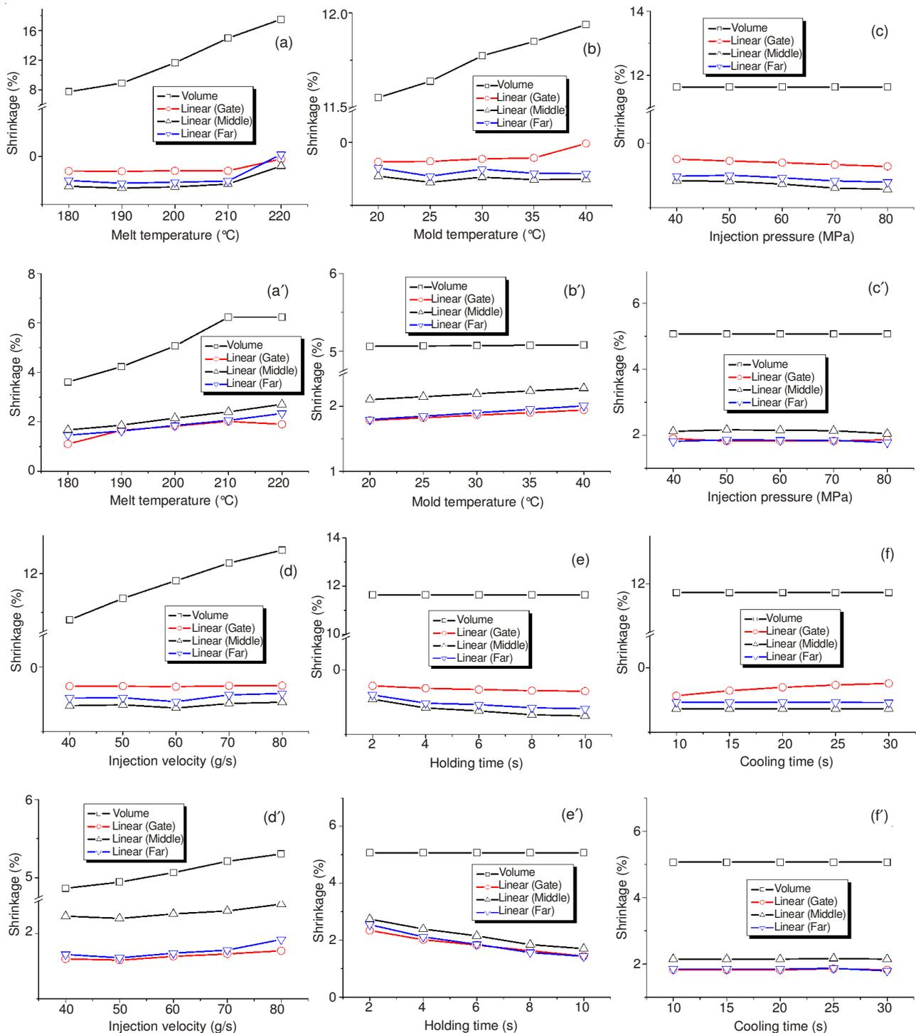
Fig. 2. Effect of operational variables on the shrinkage of PLA2. Thickness of cavity: (a-f) 1 mm, (a'-f') 4 mm
