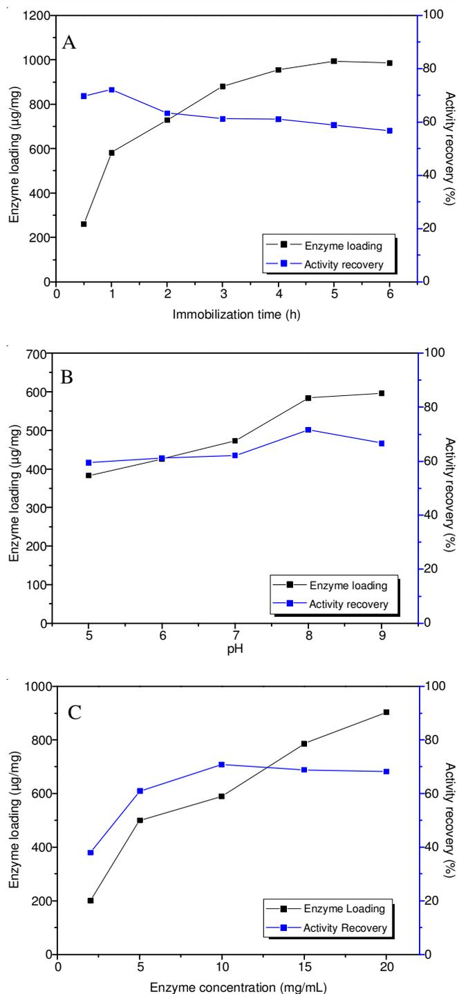
Fig. 4. Effects on alkaline protease immobilization efficiency, A immobilization's time, B pH, C enzyme concentration. Immobilization condition: 0.5 g/mL of enzyme solution per gram of support. The optimum conditions were determined weighing the enzyme loading and activity recovery
