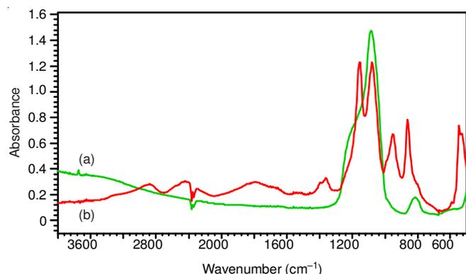
Fig. 3. Fourier transform infrared spectrum of carrier (SBA-15) and immobilized enzyme, (a) carrier, (b) immobilized enzyme. Condition: 1 mg of sample baked for 5 h at 130 °C mixed with 200 mg of KBr in disk method.
