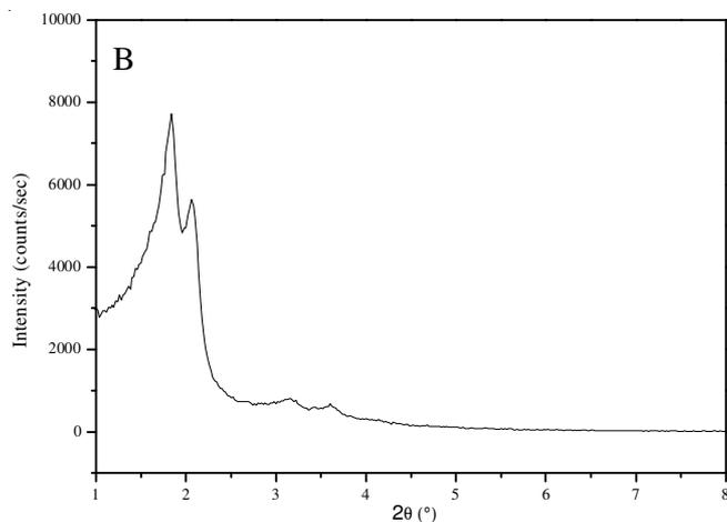
Fig. 1. Powder X-ray diffraction patterns of mesoporous materials, A SBA-15, B MCM-41
