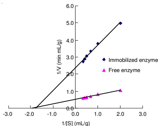
Fig. 6. Lineweaver-Burk plot for the free and immobilized enzyme. Using casein as the enzyme substrate, casein was dissolved in water containing 0.01 M NaOH
