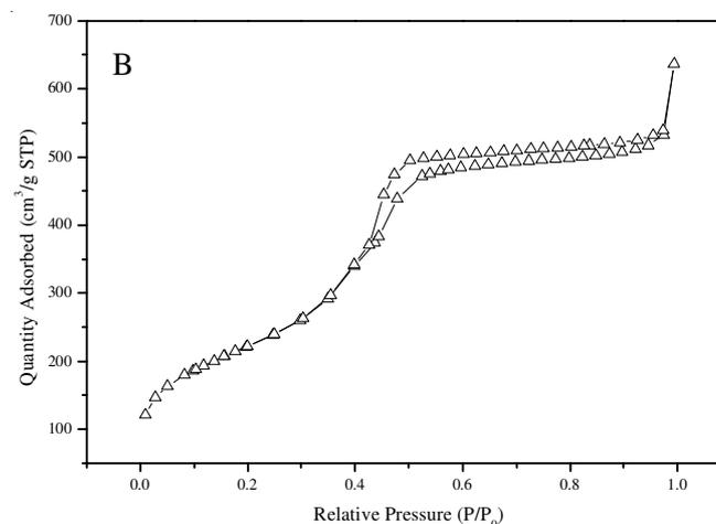
Fig. 2.  $N_2$  adsorption isotherms of SBA-15 and MCM-41, A SBA-15, B MCM-41
