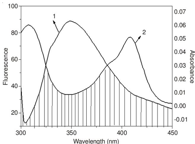
Fig. 5. Overlapping between the fluorescence emission spectrum of trypsin (1) and UV/visible absorption spectrum of brilliant blue (2).  $c$  (trypsin) =  $2.0 \times 10^{-5}$  mol L $^{-1}$ ,  $c$  (brilliant blue) =  $3.0 \times 10^{-5}$  mol L $^{-1}$ ; pH = 7.24, T = 298 K
