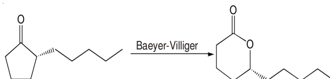
Fig. 2. Preparation of (R)- \delta -decalactone by the Baeyer-Villiger oxidation of (R)-2-alkylcyclopentanone with m -CPBA at room temperature
