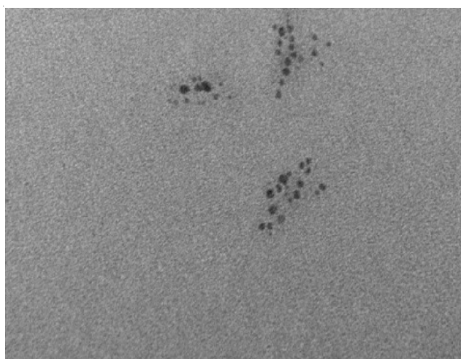
Fig. 2. TEM image of ZnO nanoparticles
