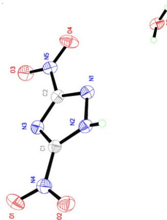
Fig. 3. Crystal structure of DNT
