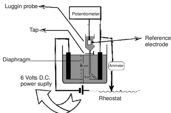
Fig. 1. Electrolytic cell and the electrical circuit
