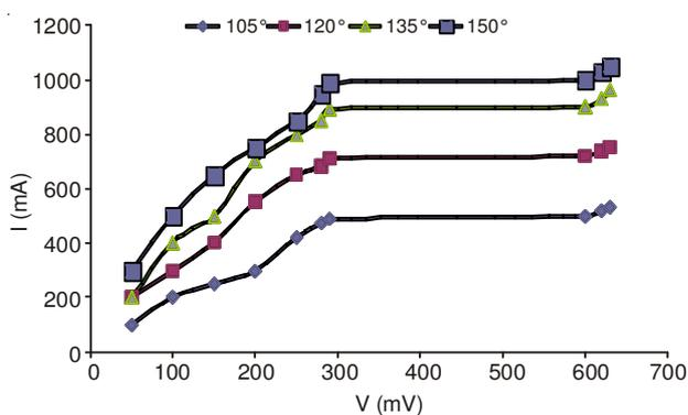
Fig. 2. Current-potential curve at different inclination, 10 cm height and 0.01 M CuSO<sub>4</sub>
