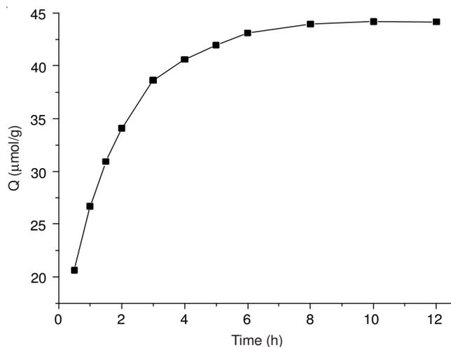
Fig. 4. Adsorption kinetics curve of molecularly imprinted polymer
