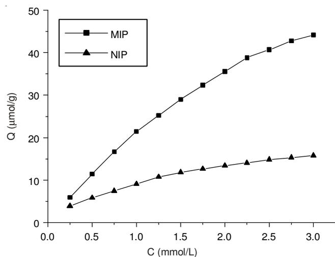
Fig. 2. Adsorption isotherms of molecularly imprinted polymer (MIP) and non-imprinted polymer (NIP)
