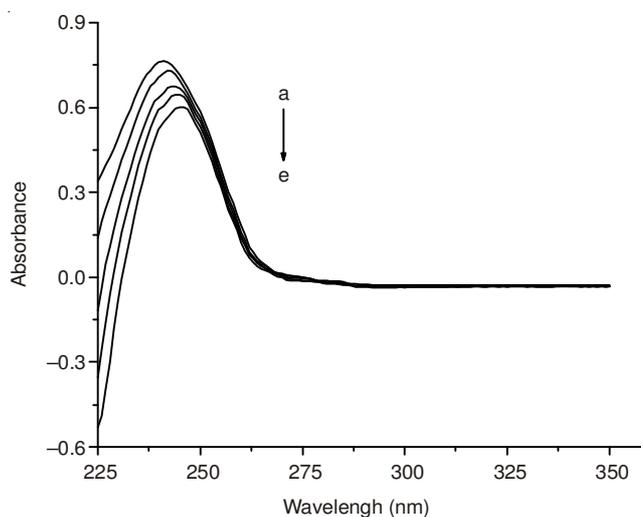
Fig. 1. UV absorption spectrum of acetanilide to different molar ratio of methacrylic acid. Curves a-e: stand for acetanilide to methacrylic acid from 1:0, 1:2, 1:4, 1:6, 1:8, in molar ratio, respectively
