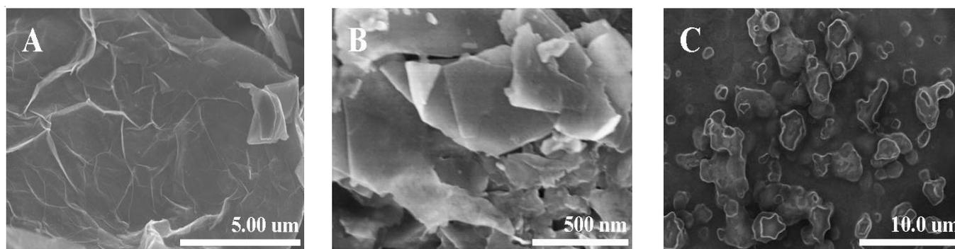
Fig. 1. Scanning electron microscope of images of graphene (a), Graphene/tetraphenylboron-dopamine complexes (b) and graphene/tetraphenylboron-dopamine/graphite electrode (c)
