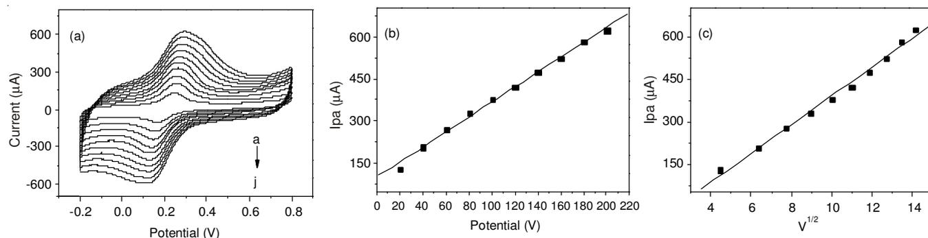
Fig. 4. Cyclic voltammograms of graphene/tetraphenylboron-dopamine/graphite electrode in 0.1 M phosphate buffer containing  $1 \times 10^{-4}$  mol/L dopamine at different scan rate (a-j): 20, 40, 60, 80, 100, 120, 140, 160, 180 and  $200 \text{ mV s}^{-1}$  (a); Graph of anodic peak current versus scan rate (b); Graph of anodic peak current versus the square root of the scan rate (c)
