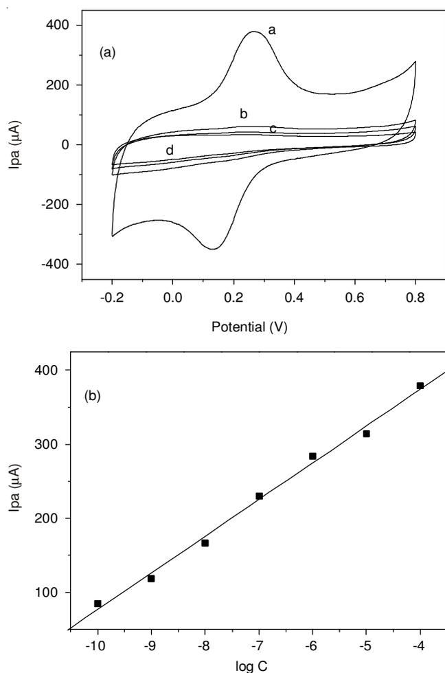
Fig. 5. Cyclic voltammograms scanned by graphene/tetraphenylboron-dopamine/graphite electrode in the presence of  $1 \times 10^{-4}$  mol/L dopamine, 0.1 mol/L ascorbic acid and 0.1 mol/L uric acid (a), 0.1 mol/L ascorbic acid (b), 0.1 mol/L uric acid (c) in 0.1 M phosphate buffer (d) at scan rate of  $100 \text{ mV s}^{-1}$  (A); Calibrating plots of the anodic peak current *versus* logarithm of the dopamine concentrations in the presence of ascorbic acid and uric acid (B)
