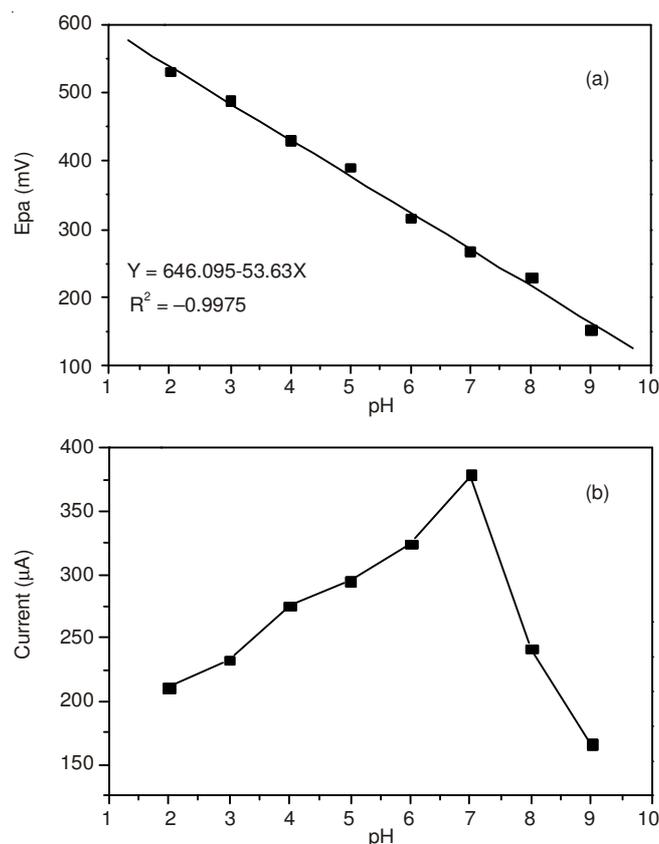
Fig. 3. Plots of variation of  $E_{pa}$  (a) and  $I_{pa}$  (b) with pH change in the concentration of  $1 \times 10^{-4}$  mol/L dopamine solution at the surface of graphene/tetraphenylboron-dopamine/graphite electrode. Scan rate:  $100 \text{ mV s}^{-1}$
