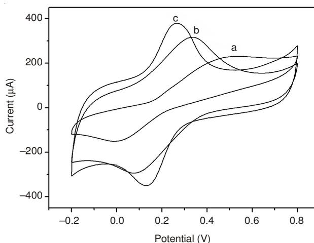
Fig. 2. Cyclic voltammograms of bare graphite electrode (a), tetraphenylboron-dopamine/graphite electrode (b), graphene/tetraphenylboron-dopamine/graphite electrode (c) in 0.1 mol/L phosphate buffer (pH 7) containing  $1 \times 10^{-4}$  mol/L dopamine. Scan rate: 100 mV s<sup>-1</sup>
