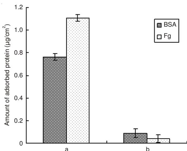
Fig. 5. Protein adsorption on the (a) virgin cover glass and (b) PMT82 modified surfaces. The bars represent the standard deviation ( $n=3$ )
