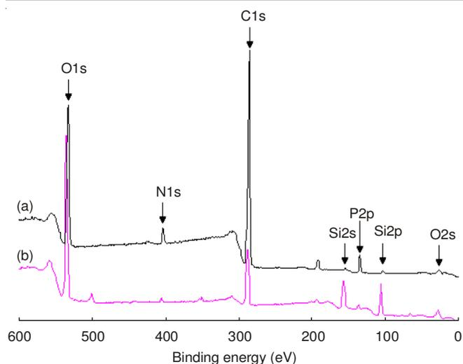
Fig. 4. XPS spectra of PMT82 coatings (a) before and (b) after DCA
