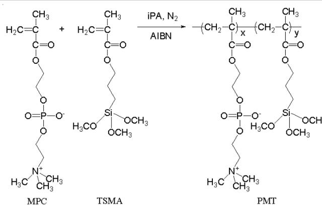
Fig. 1. Synthetic scheme of the polymer PMT
