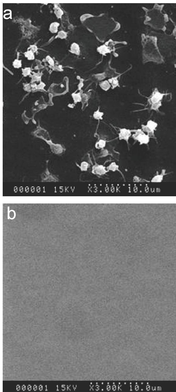
Fig. 6. SEM photographs of platelet adhesion on the (a) virgin cover glass and (b) PMT82 modified surfaces
