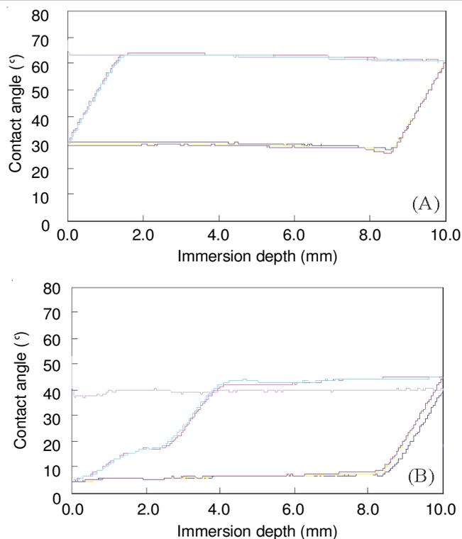
Fig. 3. Dynamic contact angle cycles of (A) cover glass and (B) PMT82 modified surfaces
