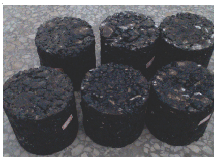
Fig. 2. Asphalt mixture specimens
