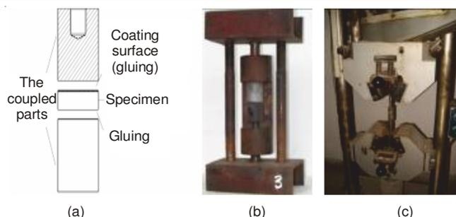
Fig. 2. Tensile test of specimen (a) Schematic of tensile test specimen; (b) Clamping process; (c) Tensile setup
