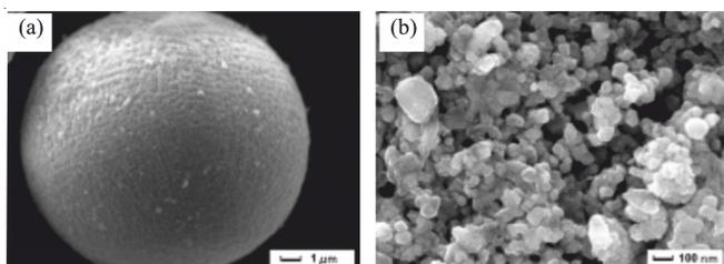
Fig. 1. Morphologies of nanostructured agglomerated powder (a) over morphology; (b) internal morphology
