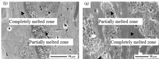
Fig. 4. SEM images of plasma sprayed nanostructured Al<sub>2</sub>O<sub>3</sub>-13 % TiO<sub>2</sub> coating (a) before optimization (#1 specimen); (b) after optimization
