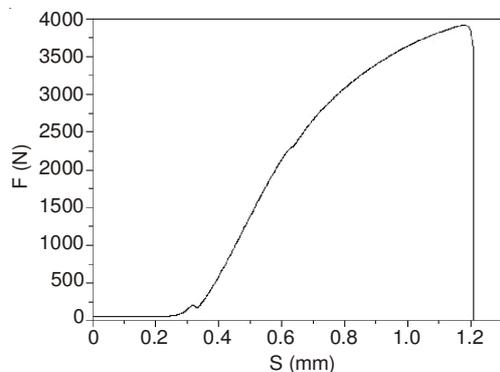
Fig. 2. Shear strength curve of the base material
