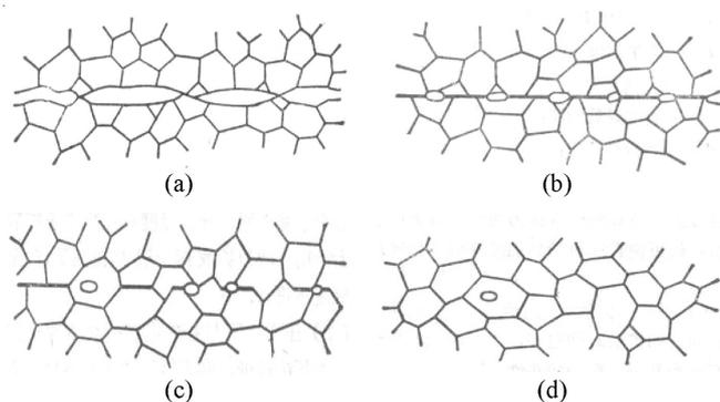
Fig. 7. Three-stage model of diffusion welding<sup>12</sup>. (a) The initial contact (b) Formation of deformation and interface. (c) Grain boundary migration and pore elimination (d) Volume diffusion and pore elimination
