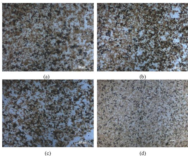
Fig. 5. Optical micrograph results of the welding seam under different holding time (500×). (a) 570 °C × 66 MPa × 3 h 1# (b) 570 °C × 66 MPa × 6 h 2# (c) 555 °C × 50 MPa × 2 h 5# (d) 555 °C × 50 MPa × 3 h 6#
