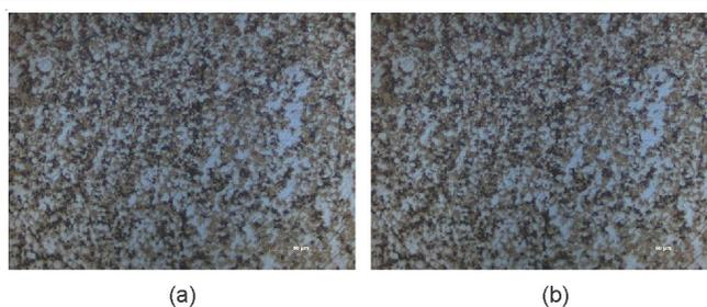
Fig. 6. Optical micrograph results of the welding seam under different holding time (500×). (a) Welding seam of specimen 7# (b) Welding seam of specimen 7# polished with 80 # sandpaper
