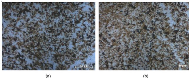
Fig. 3. Optical micrograph results of the welding seam under different welding temperature (500x) (a) 555 °C × 50 MPa × 2 h 5# (b) 570 °C × 50 MPa × 2 h 4#
