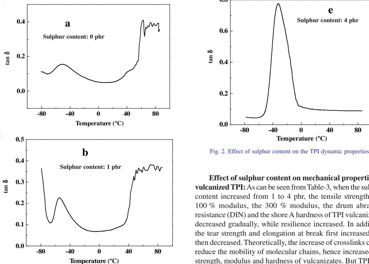
Fig. 2. Effect of sulphur content on the TPI dynamic properties
