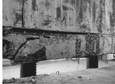
Fig. 5. Failure mode of box girder after reinforcing of CFRP
