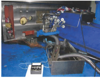
Fig. 6. Temperature rising experiment of hydrostatic bearing
