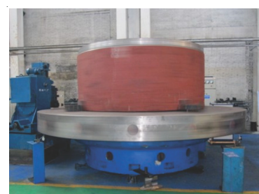
Fig. 5. Test device of hydrostatic thrust bearing system
