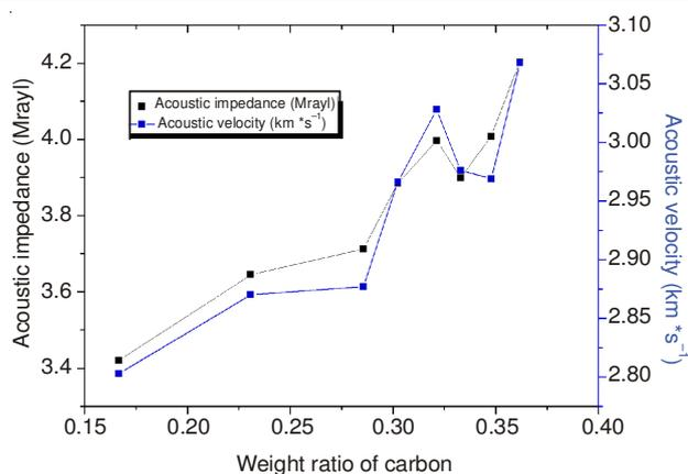
Fig. 4. Acoustic impedance and velocity of C/epoxy composite
