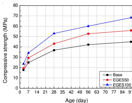
Fig. 3. Strength enhancement of concrete with EAF oxidizing slag aggregates
