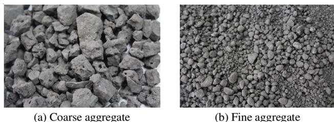
Fig. 4. View of EAF oxidizing slag aggregates
