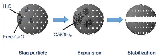
Fig. 1. Expansion mechanism of free-CaO
