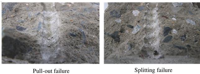
Fig. 2. Destroyed pattern specimen
