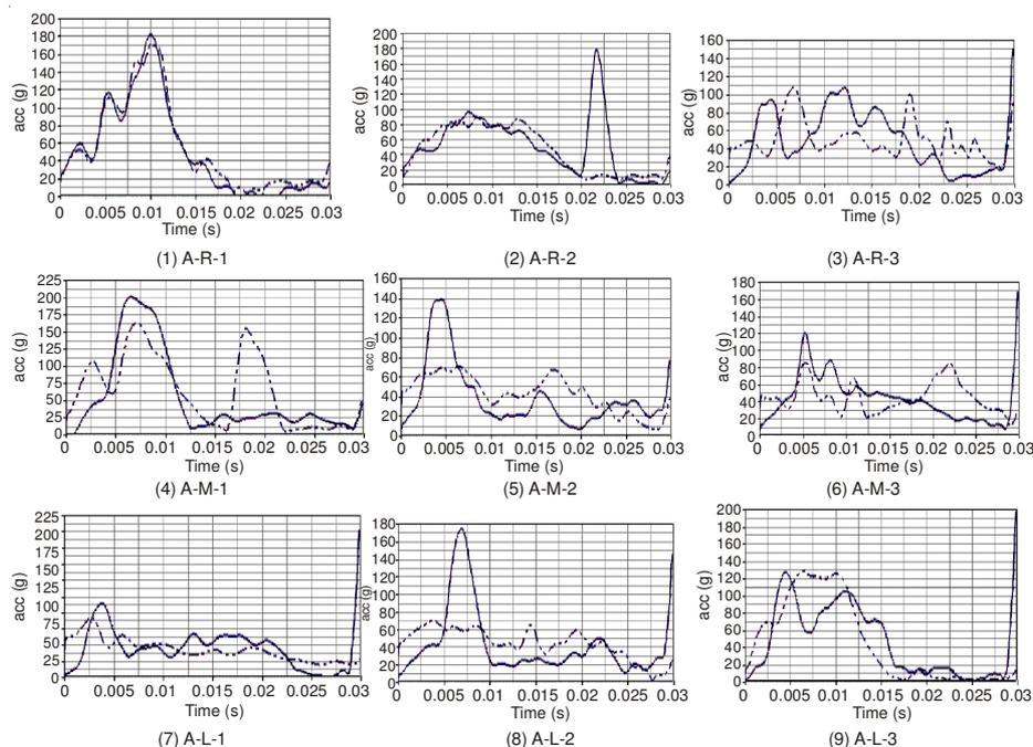
Fig. 5. Comparison of original car and modified car acceleration curves
