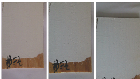
Fig. 7. Effect of the water-based coating on performance of wood board. Before experiment Soaking for 1 d in deionized water Soaking for 10 d in deionized water
