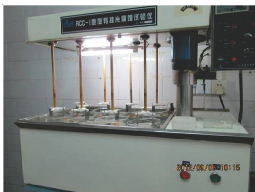
Fig. 2. Experiment testing equipments used in the rotary coupon method. (RCC-I rotary coupon corrosion rate tester)
