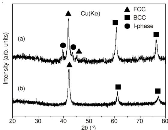
Fig. 1. XRD patterns of (a)  $\text{Ti}_{1.4}\text{V}_{0.6}\text{Ni}$  and (b)  $\text{TiVNi}$  alloys
