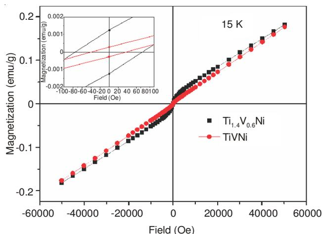
Fig. 3. Plots of magnetization of  $\text{Ti}_{1.4}\text{V}_{0.6}\text{Ni}$  alloy and  $\text{TiVNi}$  alloy as a function of applied magnetic field at 15 K
