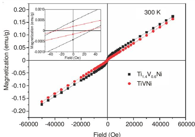
Fig. 4. Plots of magnetization of  $Ti_{1.4}V_{0.6}Ni$  alloy and  $TiVNi$  alloy as a function of applied magnetic field at 300 K (b)
