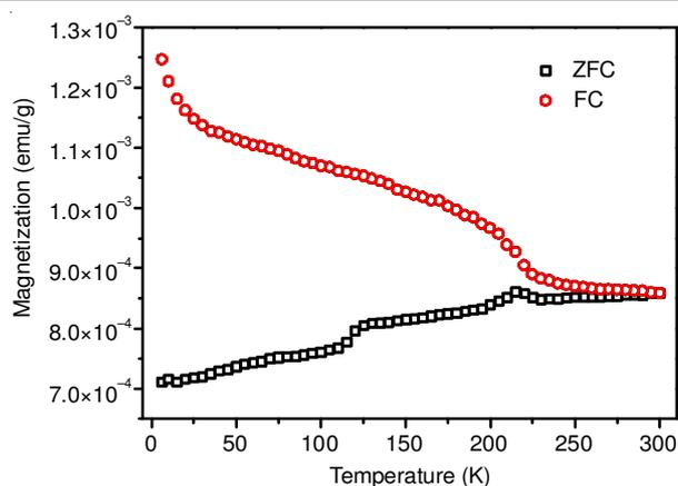
Fig. 2. Plot of magnetization of  $\text{Ti}_{1.4}\text{V}_{0.6}\text{Ni}$  quasicrystal for FC and ZFC processes at 100 Oe
