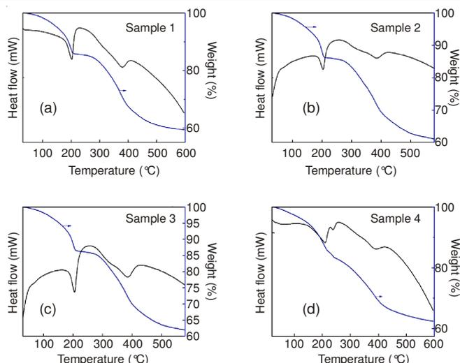
Fig. 4. TG-DTA curves of (a) sample 1, (b) sample 2, (c) sample 3 and (d) sample 4
