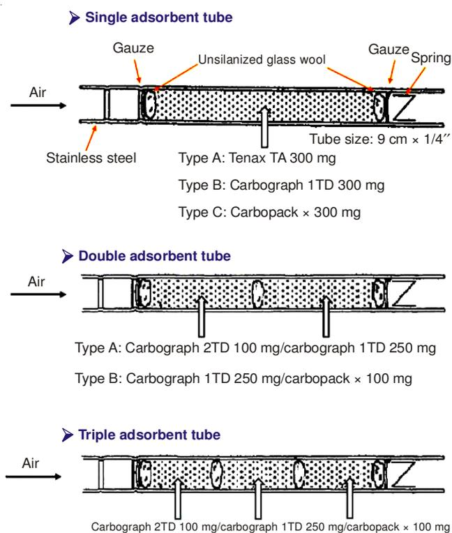
Fig. 1. Schematic diagrams of different combinations of adsorbent tubes
