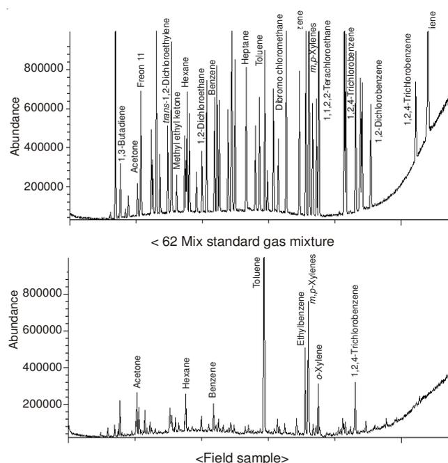
Fig. 3. Typical chromatograms of triple adsorbent tube for the standard and sample.
