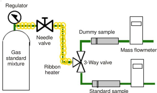
Fig. 2. Impregnation system for volatile organic compounds standard gas mixture
