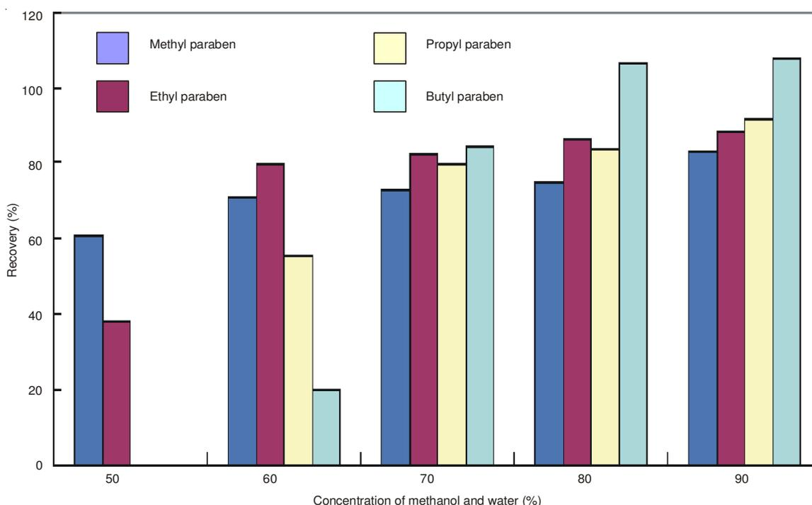
Fig. 2. Recovery of parabens (methyl paraben, ethyl paraben, propyl paraben and butyl paraben) using different concentrations of methanol (from 50 % water to 90 % methanol) as washing solution
