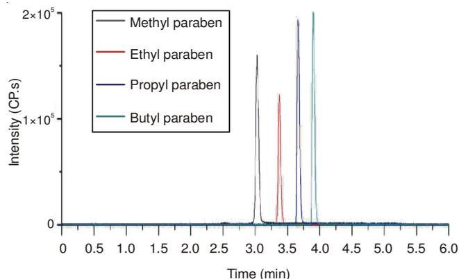
Fig. 3. Typical extracted ion chromatogram (XIC) of four parabens
